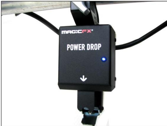
Connect the Power Drops to a 230VAC power source to check if all the Power Drops are connected. If all the Power Drops are connected in the right way all LED indicators light up.
