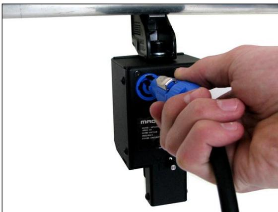
**Connect the First Power Drop with the shuko to powerCON cable.**
